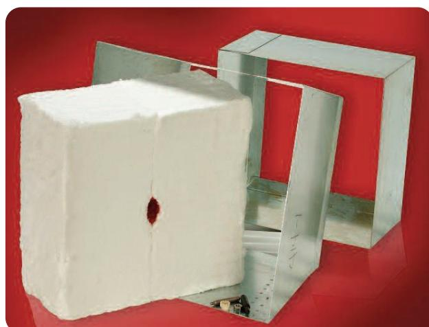
Veneering Modules are a complete system that offers a range of modules, cements, and coatings to suit specific applications. Veneering products, designed for hot face application over existing refractory linings, produce a significant reduction in heat loss through the refractory lining without requiring its replacement.
