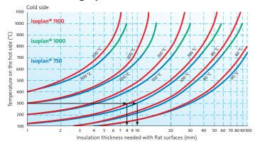
With the help of the curves in this graph, the insulation thickness needed for a specific product at defined temperatures on the "hot" and "cold" side of a flat surface can be determined.
