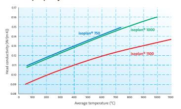
The key criterion for evaluation of an insulation material apart from high temperature resistance is heat conductivity. The heat conductivity level indicates the heat (in watts) that flows through a material 1 m thick with a surface area of 1 m² and with a temperature difference between the surfaces of 1 Kelvin (unit: W/(m·K)).
